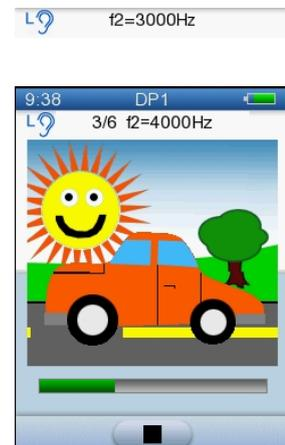
If **Child Mode** is not activated, a bar chart is displayed. See the **Test details** table below for a description of the bar chart and other data displayed.
